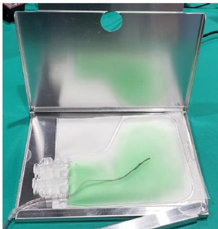
Sealed cryopreservation bag filled with 70 ml of liquid inside cassette
